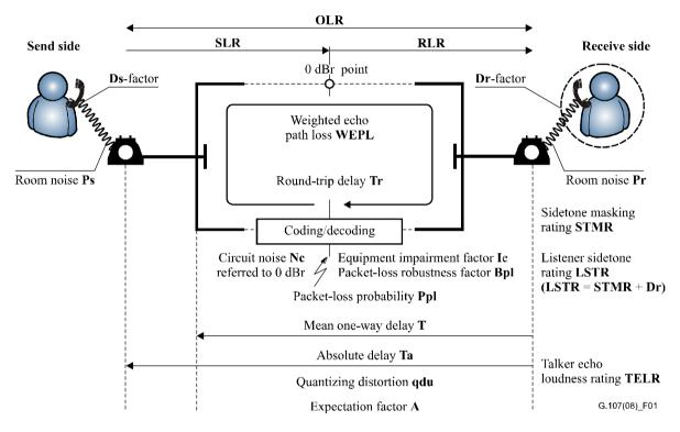
Figure 1 – Reference connection of the E-model
