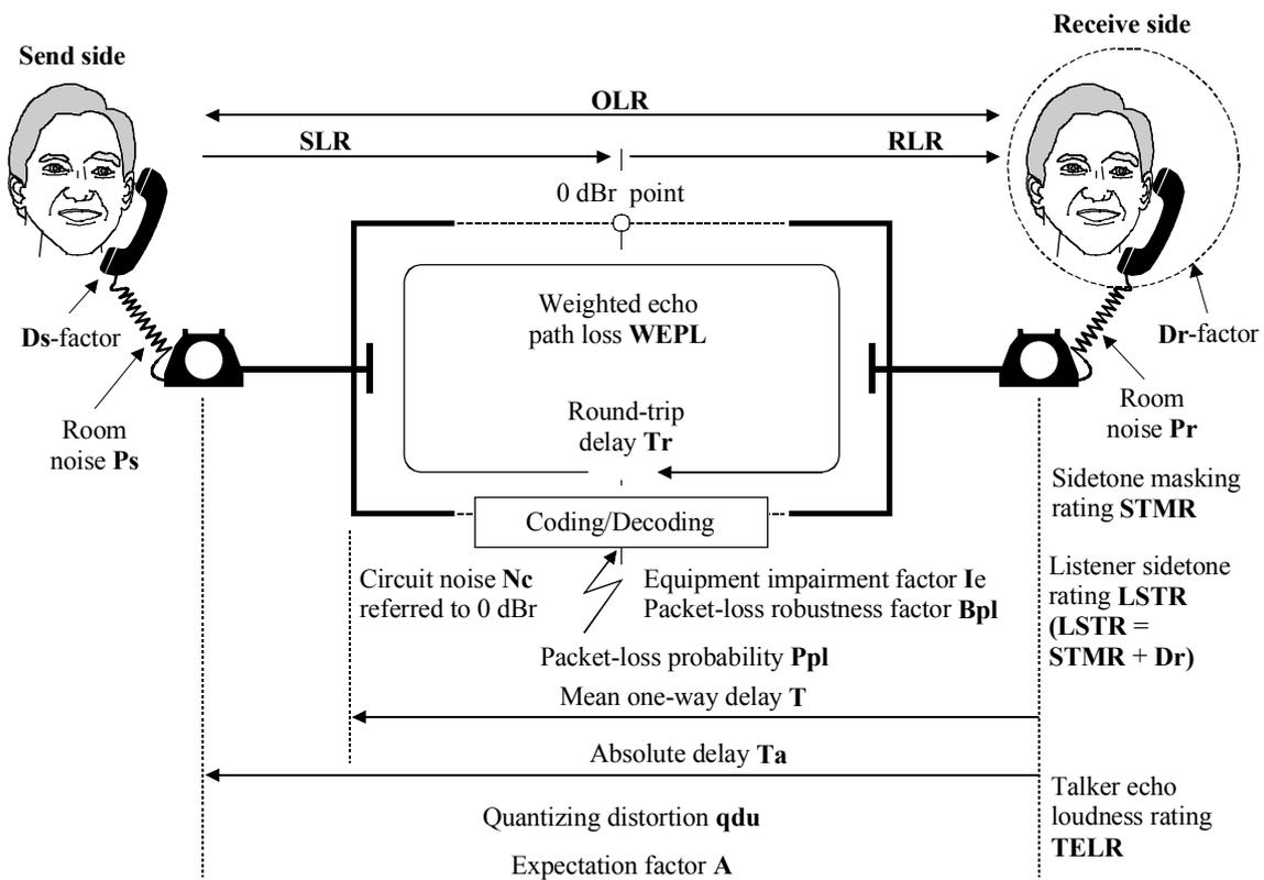
Figure 1/G.107 – Reference connection of the E-model
