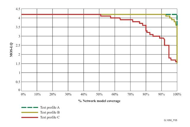
Figure 5/G.1050 – Sample network coverage curves using MOS – listening quality (100 ms jitter buffer)
