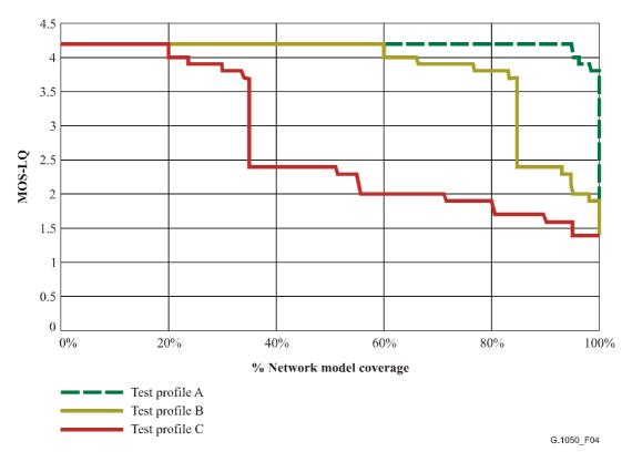
Figure 4/G.1050 – Sample network coverage curves using MOS – listening quality (40 ms jitter buffer)
