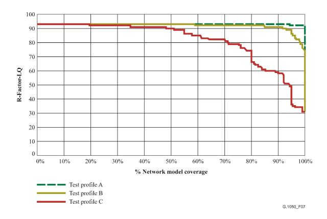
Figure 7/G.1050 – Sample network coverage curves using R-factor – listening quality (100 ms jitter buffer)
