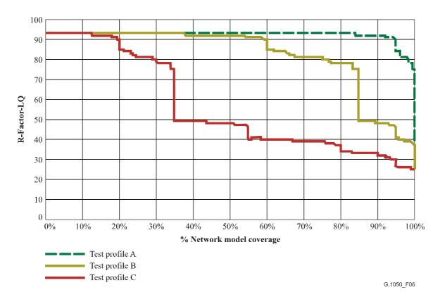
Figure 6/G.1050 – Sample network coverage curves using R-factor – listening quality (40 ms jitter buffer)
