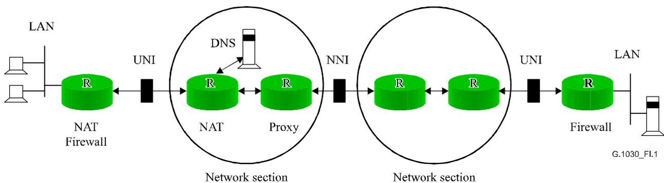
**Figure I.1/G.1030 – Reference connection with example middleboxes**
