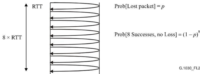
**Figure I.2/G.1030 – Handshake with 8 RT turns and no packets lost**
