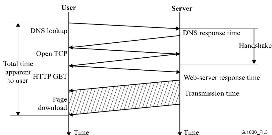
**Figure I.3/G.1030 – HTTP protocol exchange**
