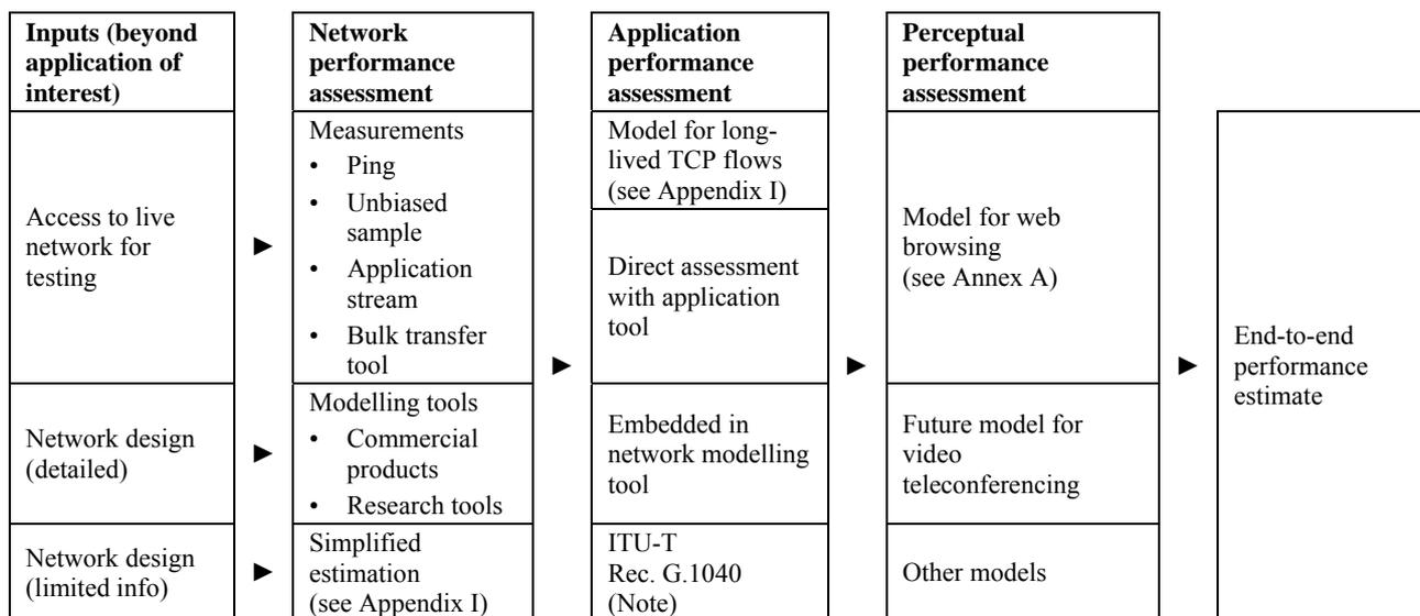
NOTE – ITU-T Rec. G.1040 provides the network contribution to transaction application performance, and does not supply the full application performance estimation, yet it gives an application-oriented view of network performance.
