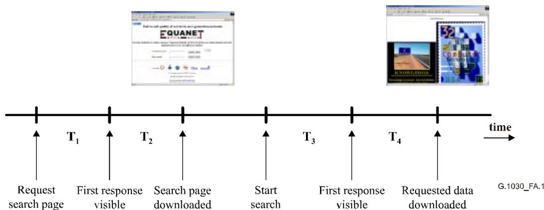
$T_1$  is the non-interactive response time and was manipulated using Java scripting.  $T_2$  is the non-interactive download time and was manipulated using the network manipulator.  $T_3$  and  $T_4$  are the equivalents for the interactive part. The sum  $T_1+T_2+T_3+T_4$  represents the session time.
