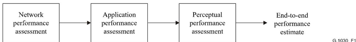
**Figure 1/G.1030 – Process to obtain end-to-end performance estimate**
