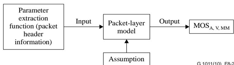
**Figure 8-2 – Packet-layer model**
