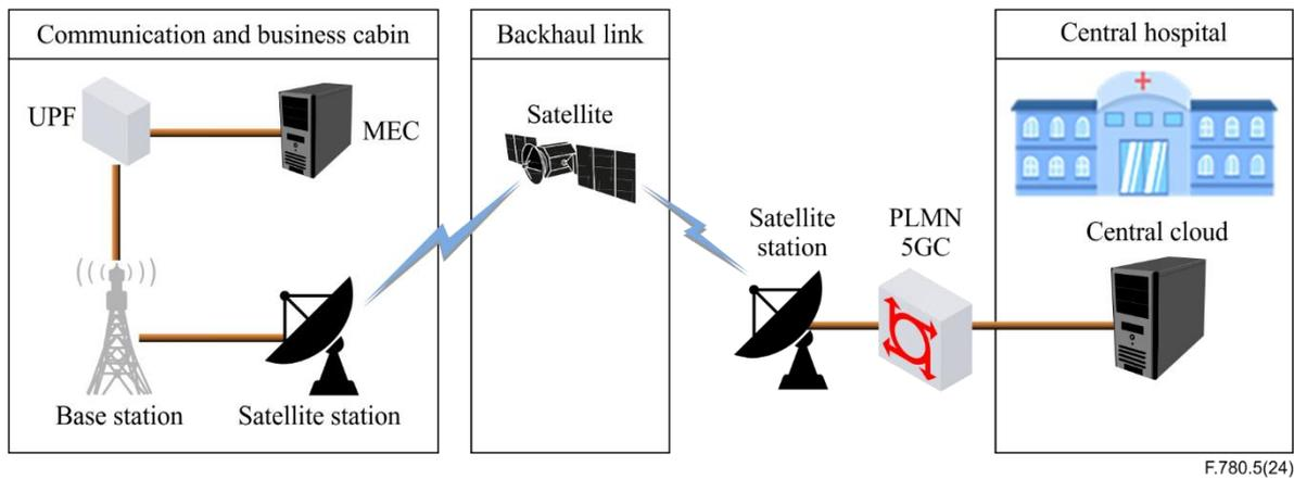
**Figure I.3 – Scenario 1: Satellite communication as the backhaul link**
