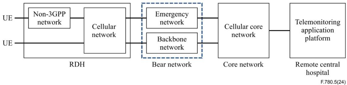
**Figure 8-2 – Reference network architecture of the network layer**
