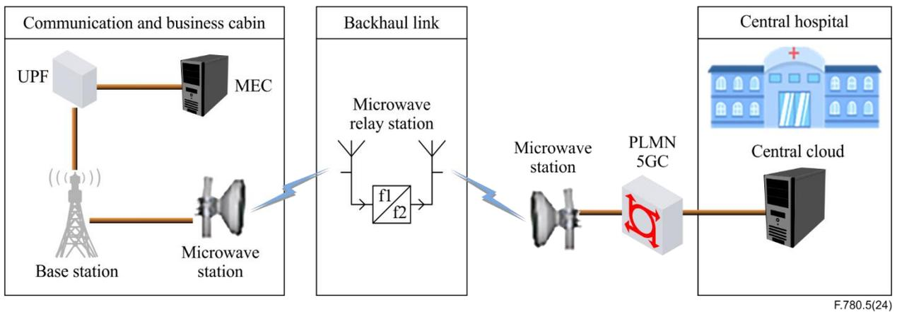
**Figure I.4 – Scenario 2: Microwave communication as the backhaul link**
