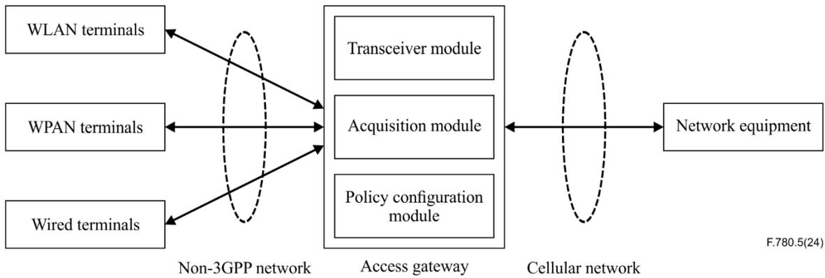
**Figure 8-4 – Reference architecture of non-3GPP network optimization**
