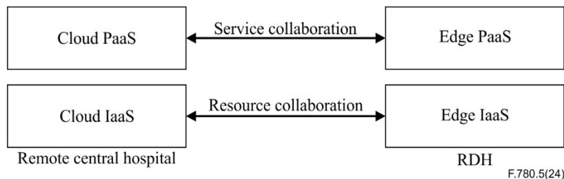
**Figure 8-5 – Reference architecture of the cloud-edge collaboration**
