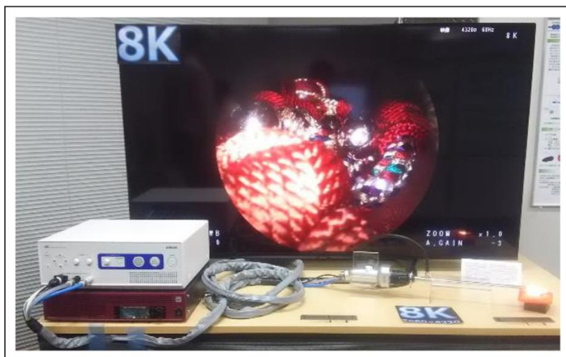
Figure II.12 – Prototype of the 8K UHD endoscope cable including a GI-POF cable, which connects the 8K UHD camera head and the CCU with a ballpoint-pen interconnection
