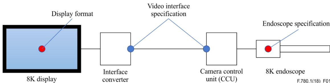
**Figure 1 – Typical configuration of a UHD endoscope system in a closed local setting**
