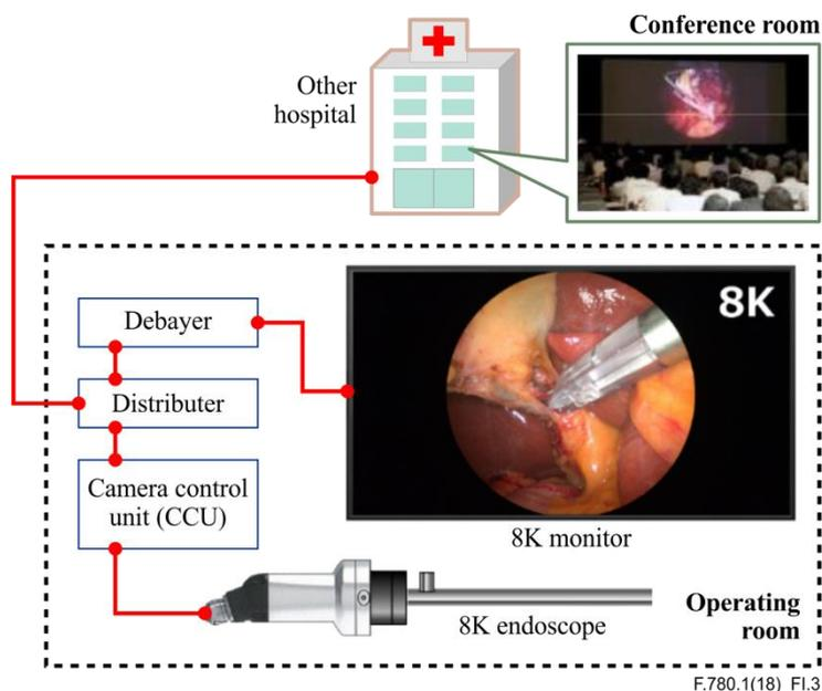
**Figure I.3 – 8K endoscope system with teleconference (remote site)**
