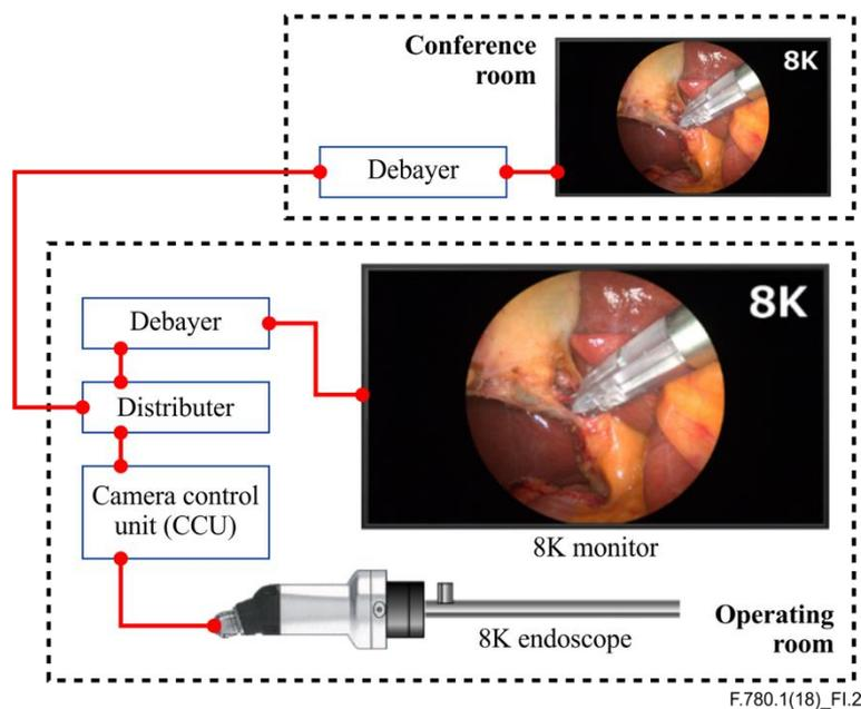
**Figure I.2 – 8K endoscope system with teleconference (in-house)**
