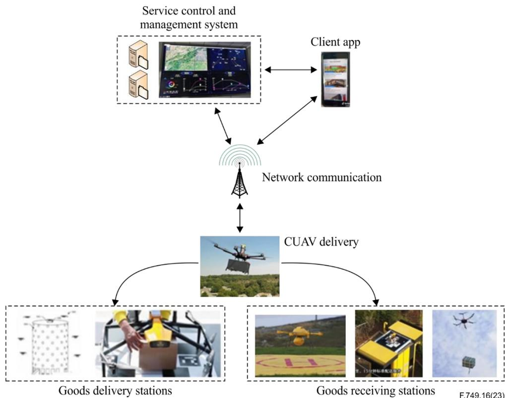
**Figure 2 – Diagram of the service procedure of CUAV logistics express delivery**
