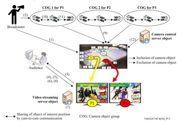
Figure I.1 – Use case for ASM broadcasting service using multi-camera objects
