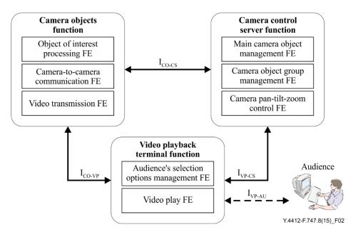
**Figure 2 – Reference architecture of ASM service framework**
