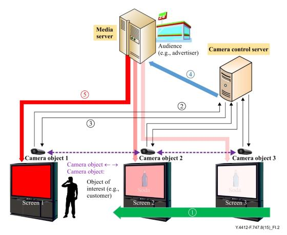
Figure I.2 – Use case for an open screen service using multi-camera objects, camera control server and media server
