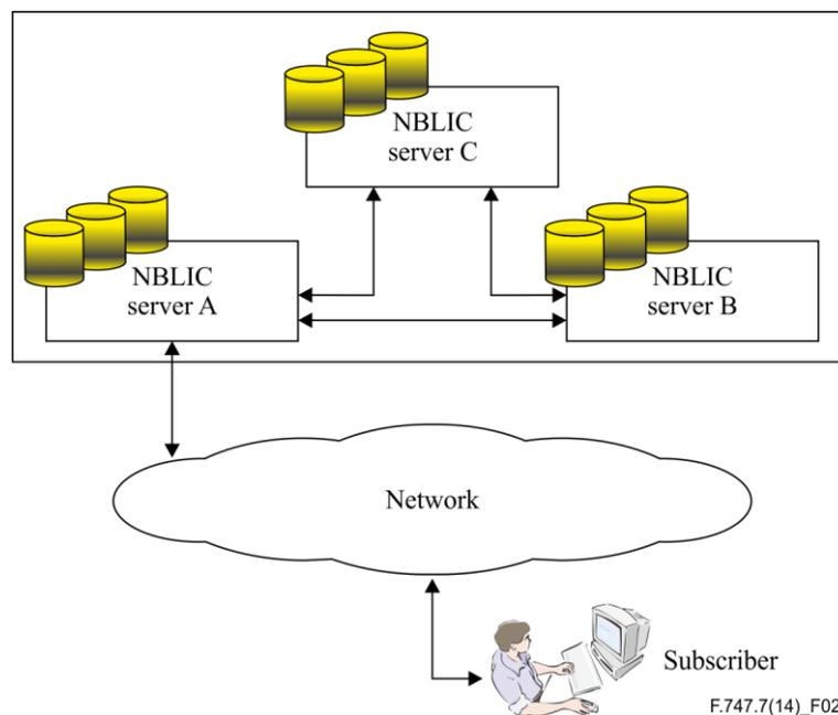
**Figure 2 – Scenario for location translation conversion using NBLIC services via a decentralized model**
