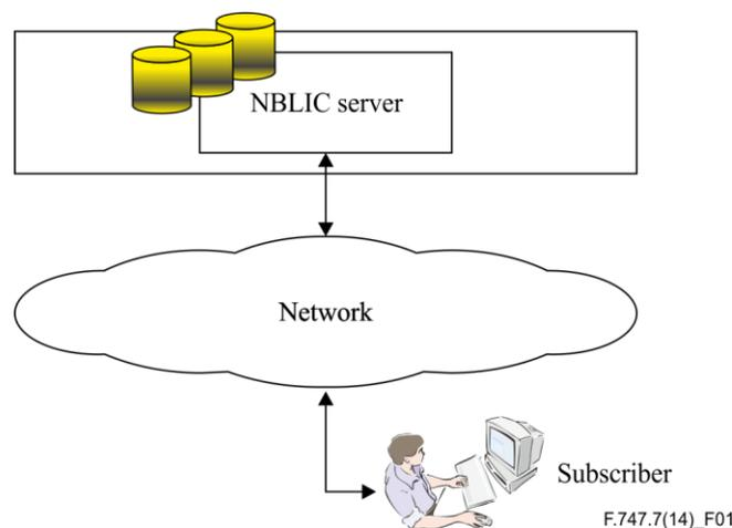
**Figure 1 – Scenario for location translation conversion using NBLIC services via centralized model**
