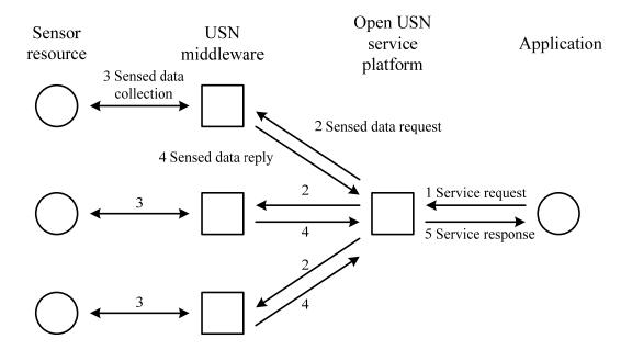
Figure 6-2 – Heterogeneous USN middleware access through the open USN service platform
