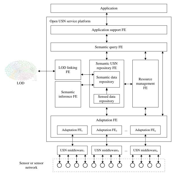
Figure 8-1 – Functional architecture of the open USN service framework
