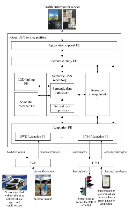
Figure II.1 – Traffic information service using the open USN service platform
