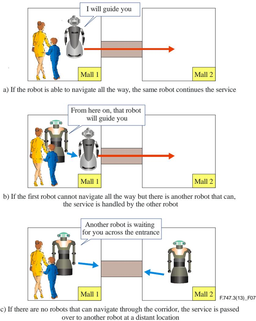
**Figure 7 – Example of service handover between robots**
