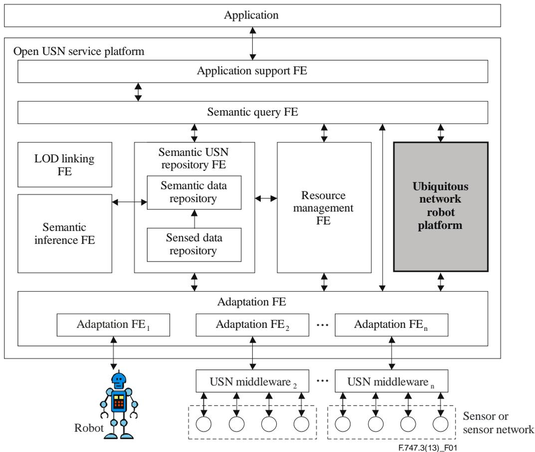
**Figure 1 – Relation between open USN service platform and UNR-PF**
