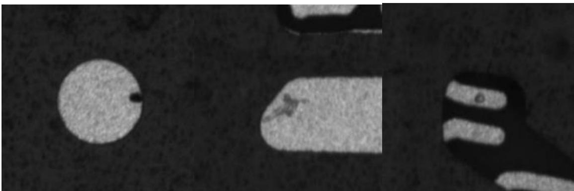
**Figure I.5 – Illustrations of defects (lost, impurity and pit) in the semiconductor industry**
