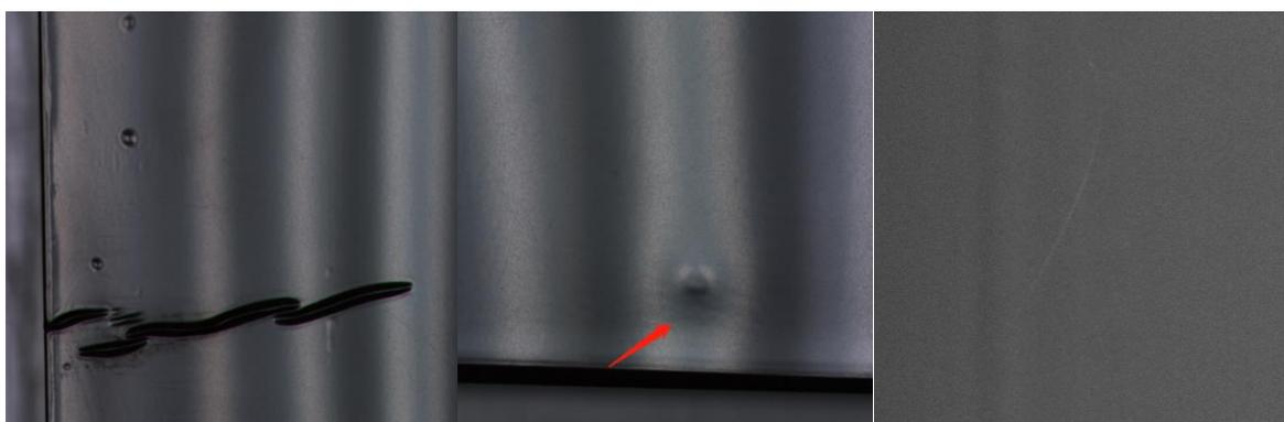
**Figure I.2 – Illustration of defects (wrinkle, pit and scratch) in the battery industry**
