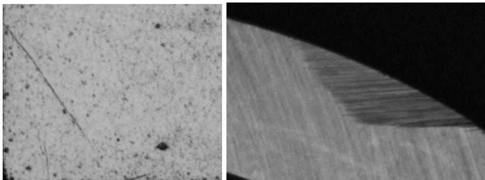
**Figure I.1 – Illustrations of defects (crack and pit) on steel products**
