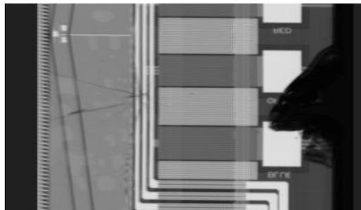
**Figure I.4 – Illustration of defects (crack and breakage) in the display industry**
