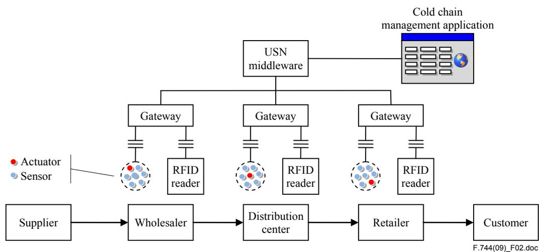
**Figure 2 – Use case of a cold chain management service**
