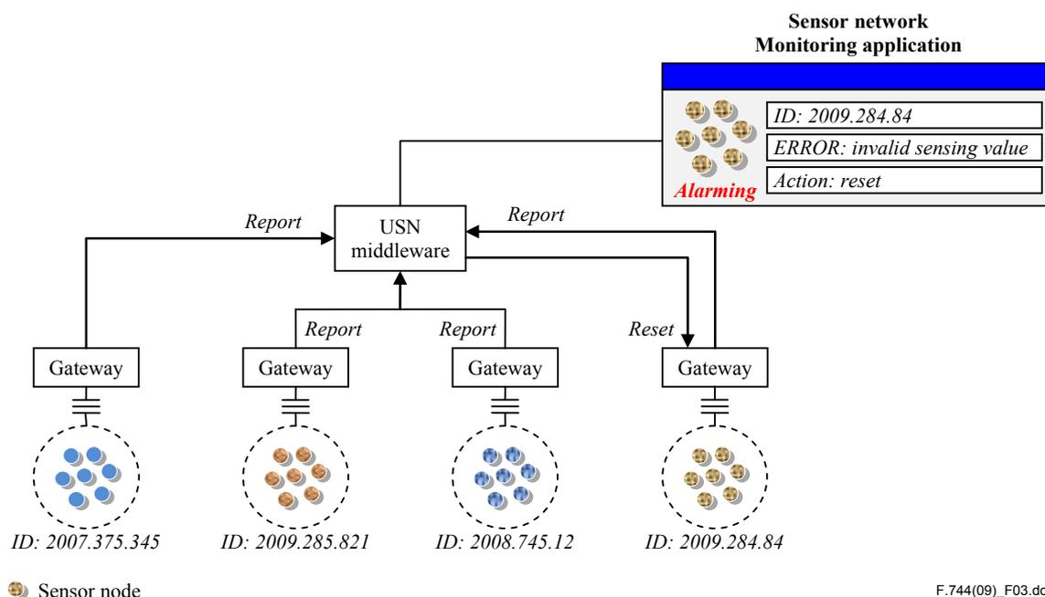
**Figure 3 – Use case of a sensor network monitoring service**
