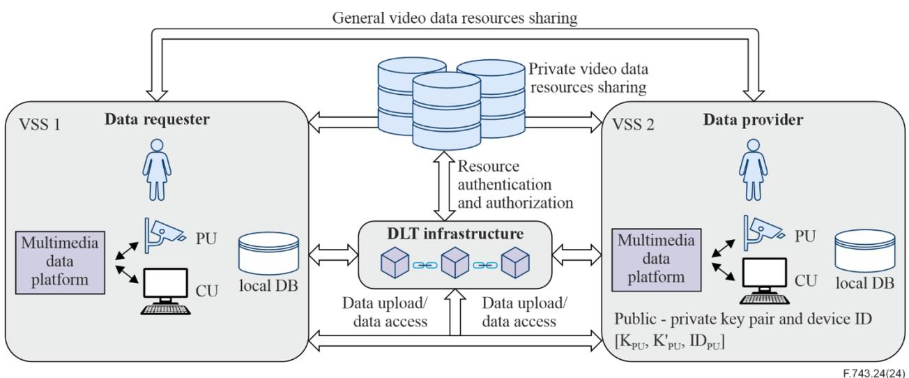
Figure 2 – General framework of DLT in video surveillance system interworking
