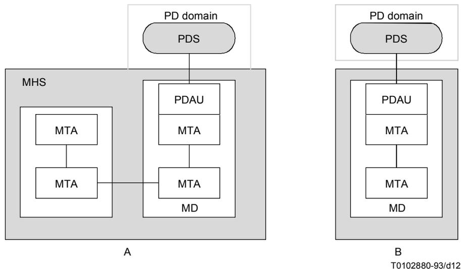
**Figure 12/F.400/X.400 – Configurations for MH/PD service intercommunication**
