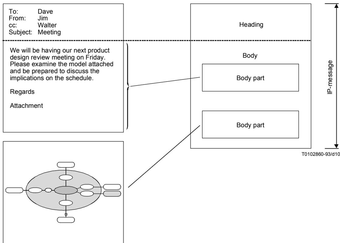
Figure 10/F.400/X.400 – IP-message structure for a typical memo
