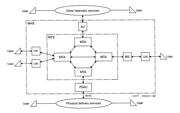
Note – Message input from PD Services to MHS is for further study. Flow from PD Services to the PDAU shown is for notifications.
