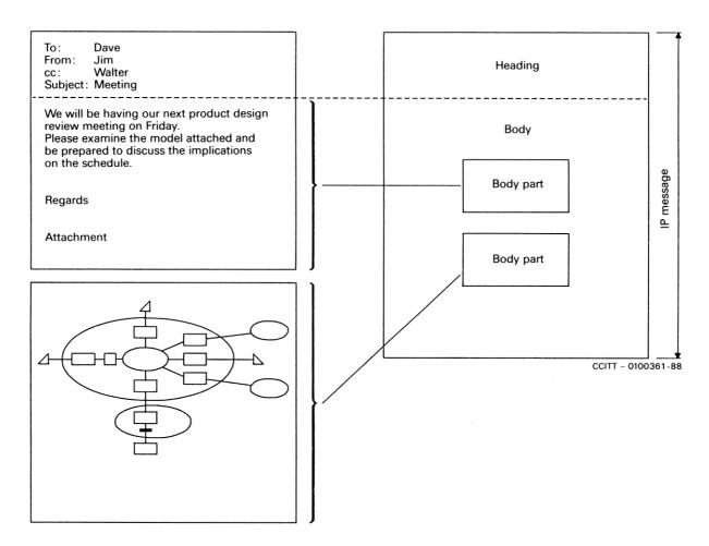
FIGURE 9/F.400 IP-message structure for a typical memo
