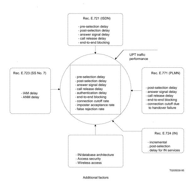
FIGURE 1/E.776 **Approach for evolving UPT traffic performance parameters**
