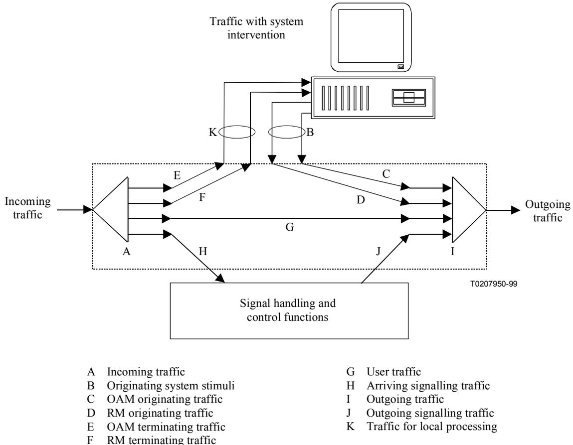
**Figure 2/E.745 – Main traffic flow diagram at an B-ISDN switch**
