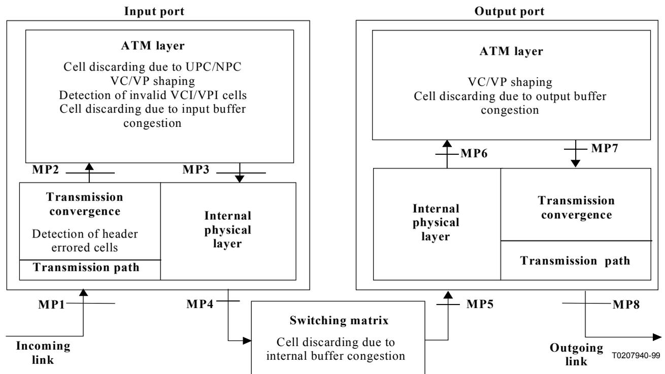
Figure 1/E.745 – Measurement points (MPs) inside the network element
