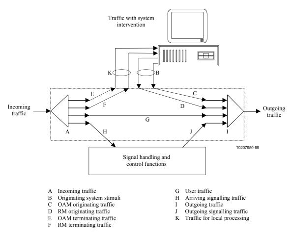
Figure 2/E.745 – Main traffic flow diagram at an B-ISDN switch
