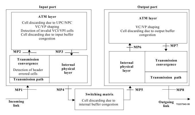
Figure 1/E.745 – Measurement points (MPs) inside the network element
