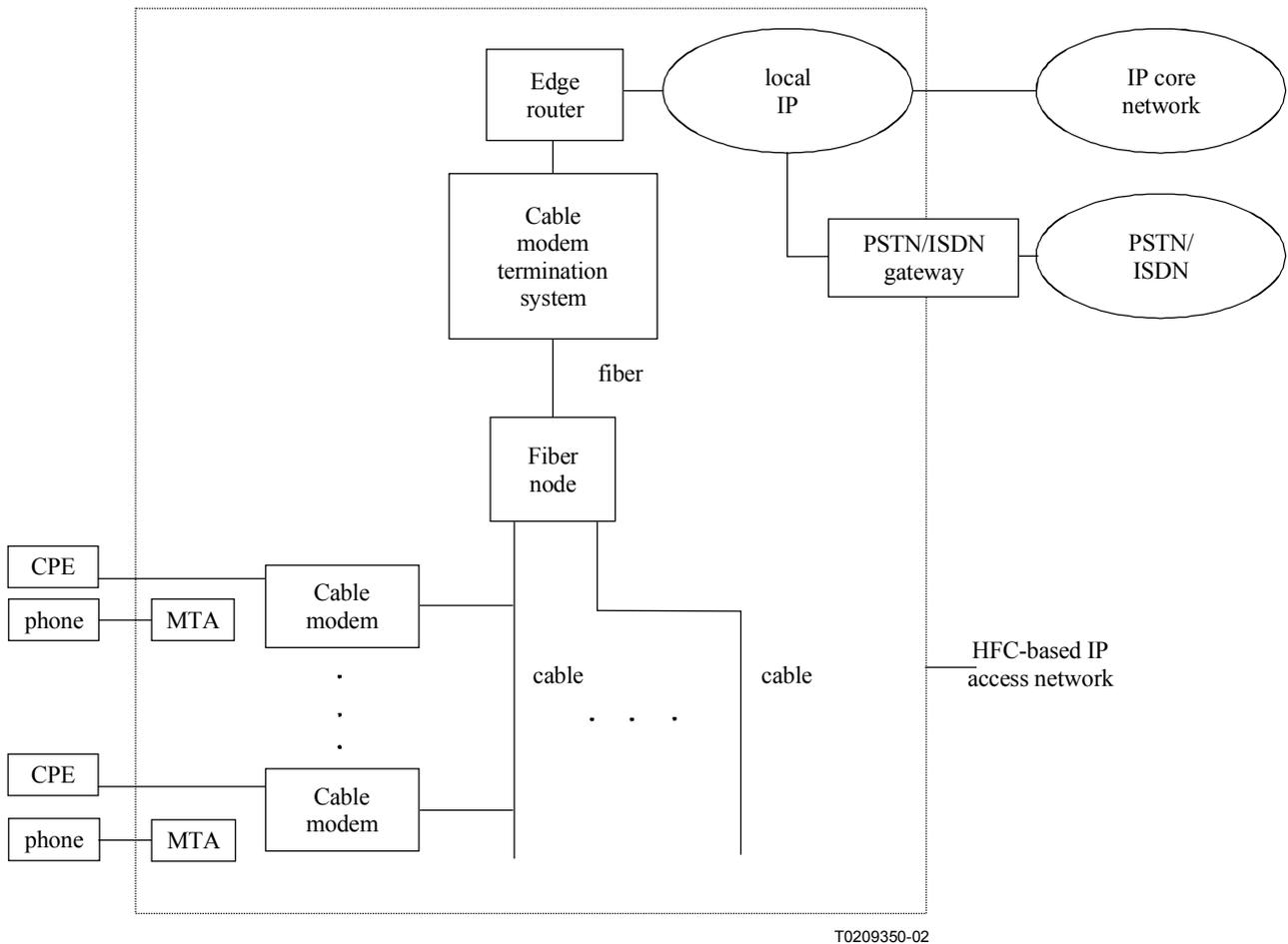
**Figure 5-1/E.681 – Reference architecture of an HFC-based IP access network**
