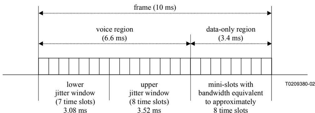
Figure II.1/E.681 – Example frame structure with two jitter windows
