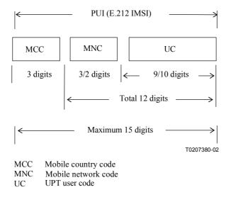
Figure 8/E.168 – Structure of the PUI in accordance with Recommendation E.212
