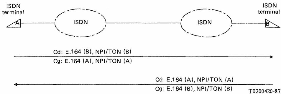
*Note 1* – This scenario represents the case of generic ISDN terminals which support NPI/TON features defined in Recommendation Q.931 and are capable of supporting all ISDN services per I-Series Recommendations.
