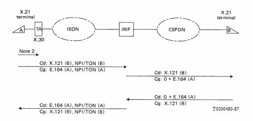
Note 1 - It is understood that the signalling protocol mapping function implemented in the X.30 TA will support the NPI/TON feature as defined in Recommendation Q.931.
