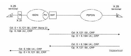
Note 1 - The PH is required to remove and insert escape code digit(s) as appropriate.
