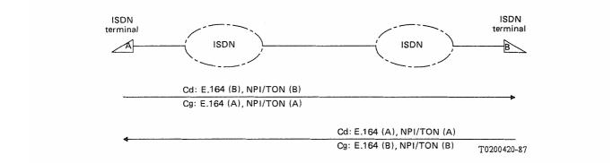
Note 1 – This scenario represents the case of generic ISDN terminals which support NPI/TON features defined in Recommendation Q.931 and are capable of supporting all ISDN services per I-Series Recommendations. Note 2 – In the short term, the NPI/TON capabilities are not available in the X.25 protocol used to handle packet mode calls. Work is in progress to provide NPI/TON in X.25.
