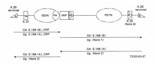
Note 1 - The PSTN terminal (B) may receive the calling party (A) number if appropriate signalling and terminal functionality is available. Note 2 - For calls originated in the PSTN, the calling number (B) may not be provided to the called terminal (A).
