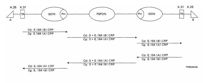
Note 1 - Meaning of abbreviations are given in § 5.5. Note 2 - The ISDN PHs are required to insert and remove escape code digits as appropriate.
