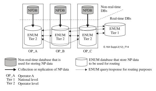
Figure 14 – Example of an ENUM technology utilization for Solution E
