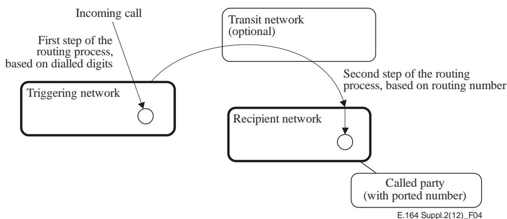
**Figure 4 – Conceptual framework for number portability (NP) handling**
