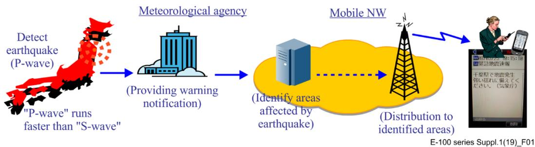
**Figure 1 – Tsunami Mobile Early Warning System Japan**
