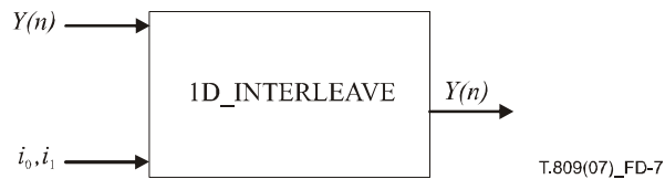
Figure D.7 – Parameters of the 1D_INTERLEAVE procedure
