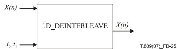
Figure D.25 – Parameters of the 1D_DEINTERLEAVE procedure
