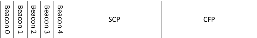
Figure B.8 – Structure of a MAC Frame
