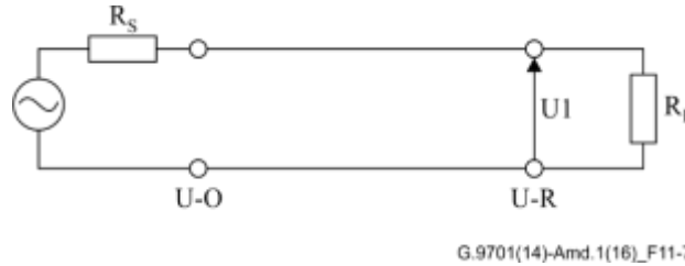
Figure 11-7 – Voltage across the load without access cabling
