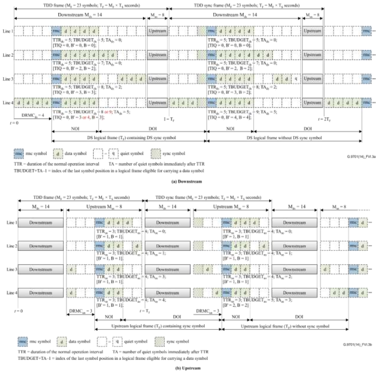
Figure VI.3 – Example 2: Avoiding common symbol periods in DOI to turn off crosstalk cancellation processing
