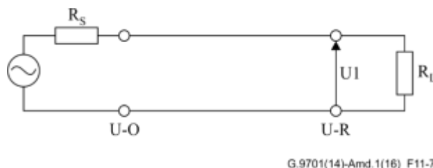
Figure 11-7 – Voltage across the load without access cabling
