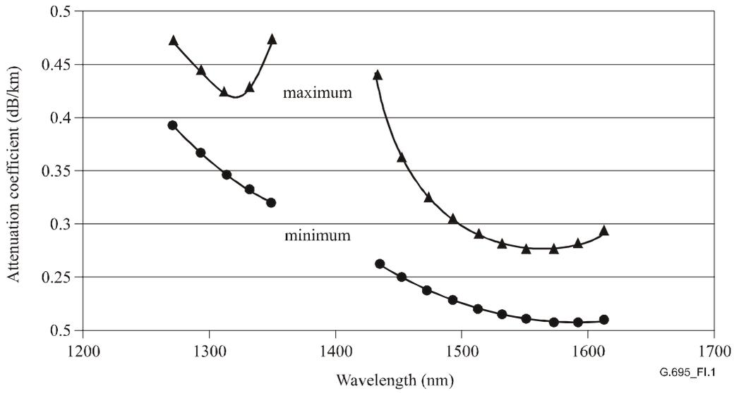
Replace **Figure I.2/G.695** – Assumed attenuation coefficient values for G.652.C&D cable by the following to show the missing markers:
