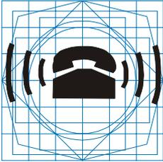
A black pictogram of a telephone handset with sound waves emanating from it, set against a blue grid background. | <p><b>Application:</b><br/>On telecommunications equipment, to indicate the control for a telephone ringing sound, or the status that the signal is calling.</p> |
