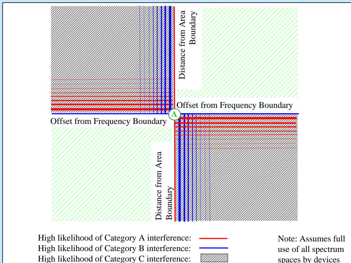
Figure 2 : Illustration of the likelihood of the three categories of interference
