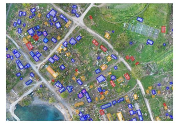
Note: Red structures are heavily damaged, blue structures moderately damaged, and yellow structures undamaged. Source: Matt Irwin, "Mapping Cyclone Pam's destruction with drones."
