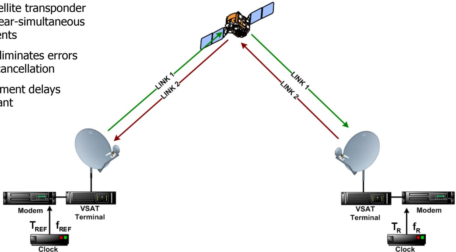
$$T_R - T_{REF} = \frac{1}{2} \left[ \left( M_{(R-REF)} - M_{(REF-R)} \right) - \left( \delta t_{Ref\ receiver} - \delta t_{R\ receiver} \right) \right]$$
