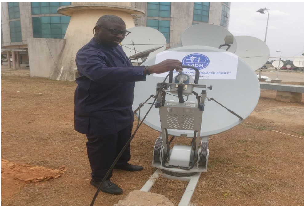
Appendix F: Mobile 1.2m Composite Ku-Band Reflector with Circular Hand Crank for Emergency/Manual Stow of Azimuth and Elevation Axes integrated with Ku-band 4W BUC and LNB undergoing series of tests before deployment in Internal Displaced Persons (IDP) camps.
