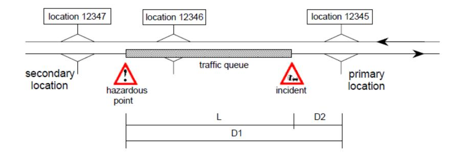
With PLR offsets on the TMC table you are able to specify the location of an incident, between TMC location nodes.
