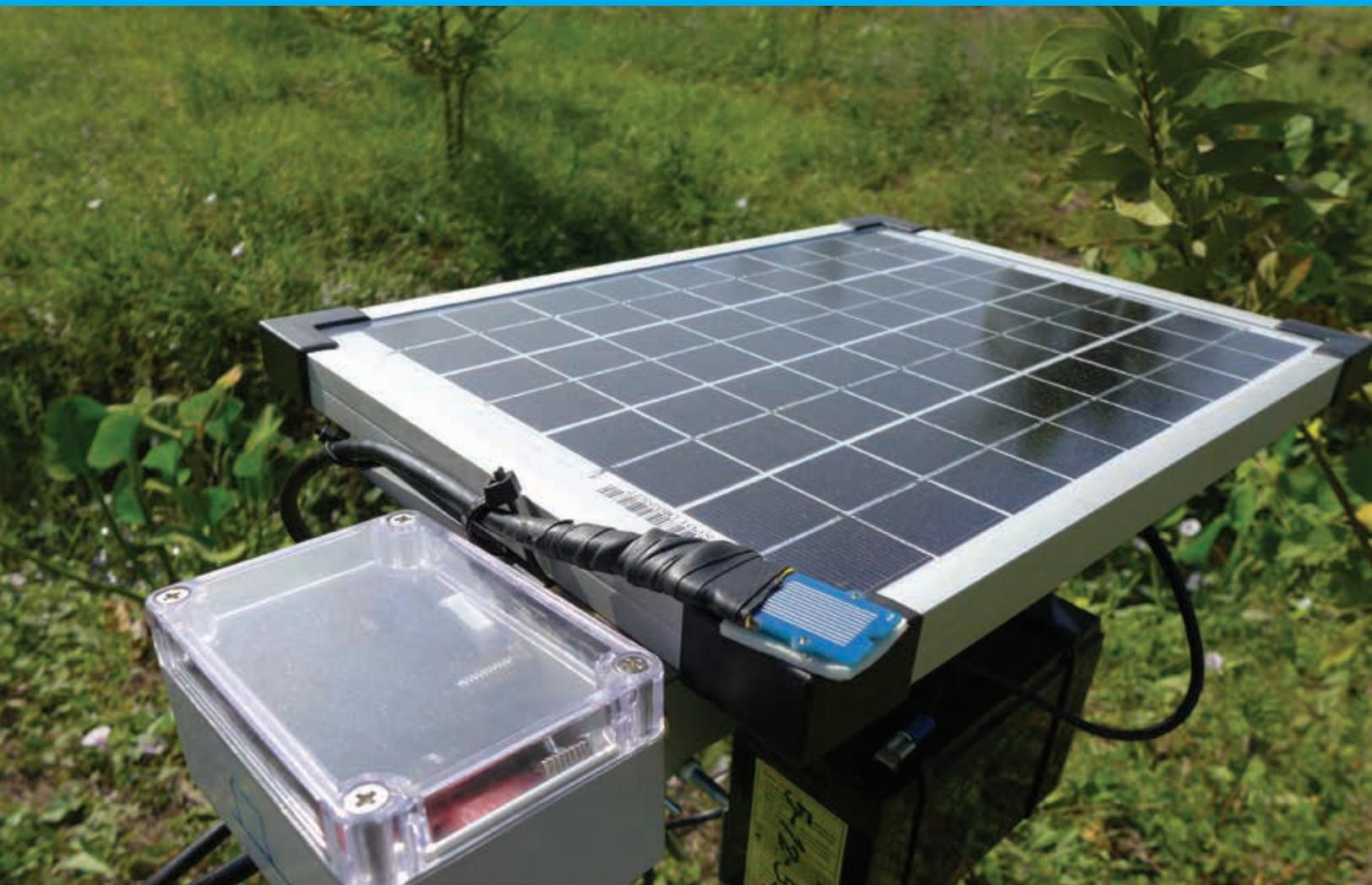
Photo credit: Marco Zennaro. Solar-powered, Wi-Fi enabled soil moisture node at the Asian Institute of Technology in Bangkok.
