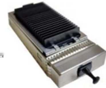
QKD Receiver module (QRx) Plugged in cage, with heat sink
