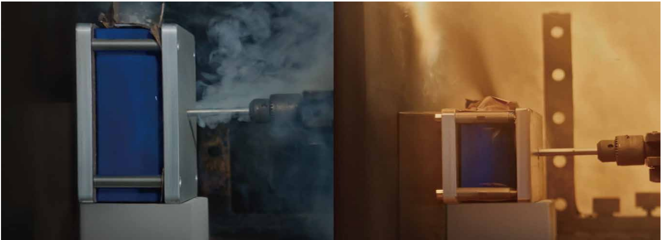
Figure 16 Lithium battery crush test:
