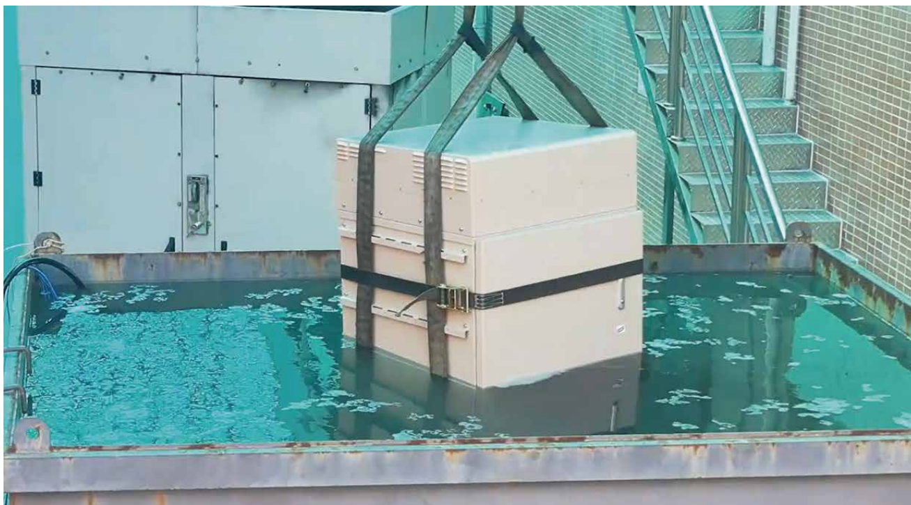
Figure 17 Lithium battery immersion test in seawater
