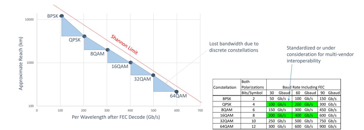
Probabilistic Constellation Shaping - Variable rate / reach tradeoff OTUCn-M provides a way to describe the information carried over a proprietary signal format in a standardized way, including the how the clients are mapped into the digital bit-stream
