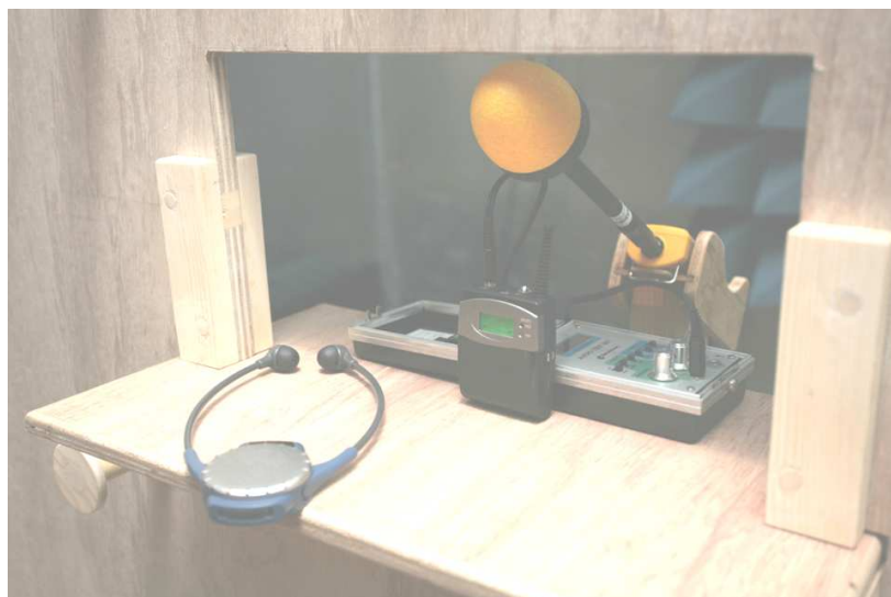
Figure 2: A tour guide system comprising of transmitter (square black device) and receiver (blue headphones with integral receiver) during test preparation. The 1 kHz tone generator can be seen behind the transmitter, and a NARDA field strength probe can be seen behind that.
