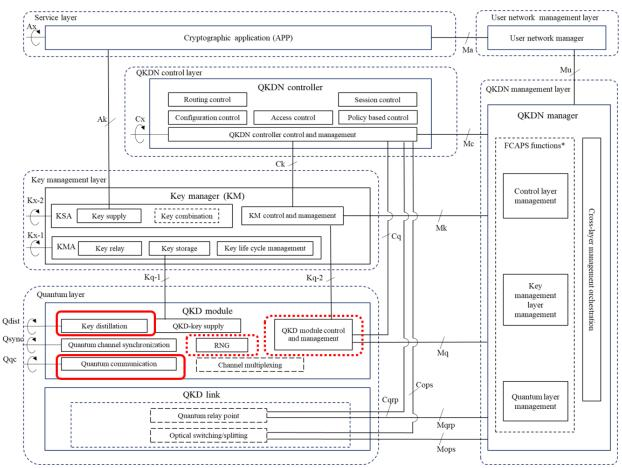
NOTE - The scope of this report covers key distillation and quantum communication module (solid red line); parameters reported to QKD control and management module and assumption for RNG (dotted red line).
