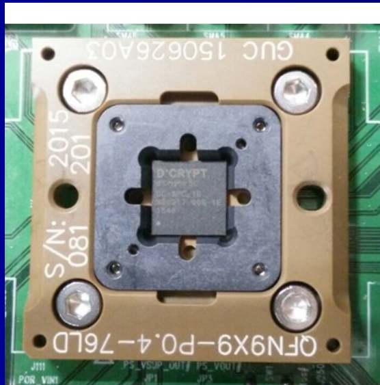
d'Cryptor SC in a test-socket
