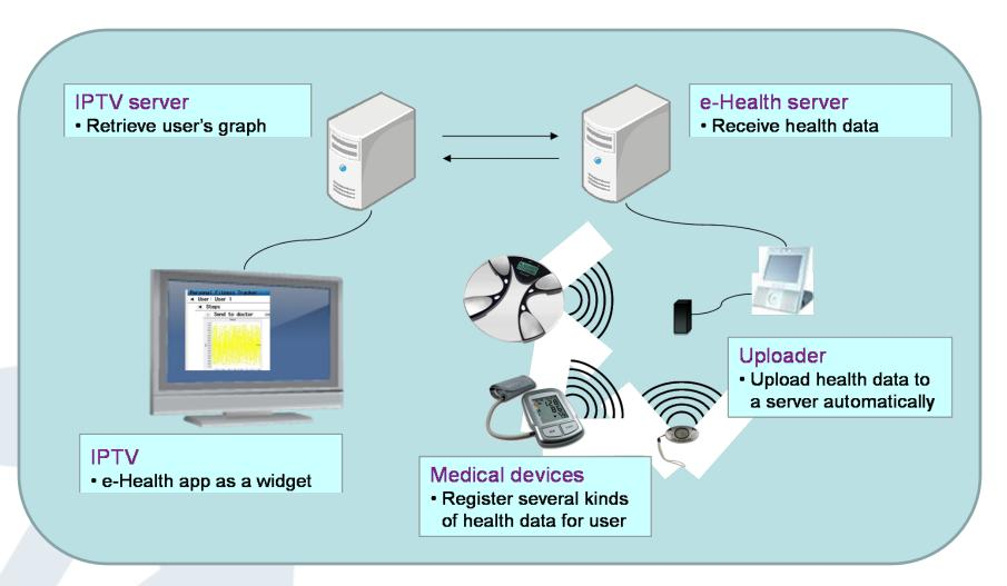
SEMI system setup showing relationship between IPTV set-top-box, e-Health server and various connected e-Health devices.
