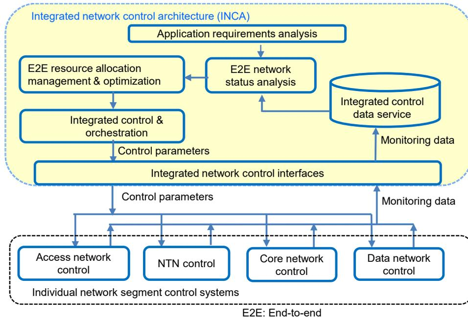
Figure 1 - TN-NTN integrated network control architecture (ITU-T Y.3207).
