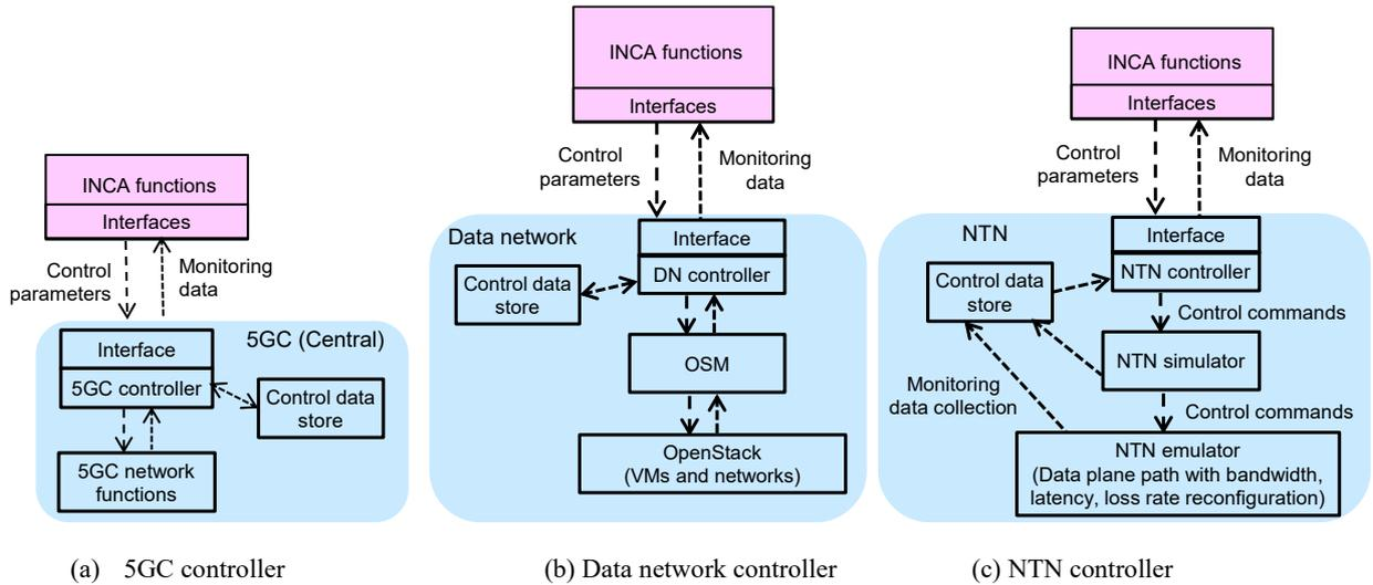
Figure 3 - Layout of 5GC, data network and NTN controllers.
