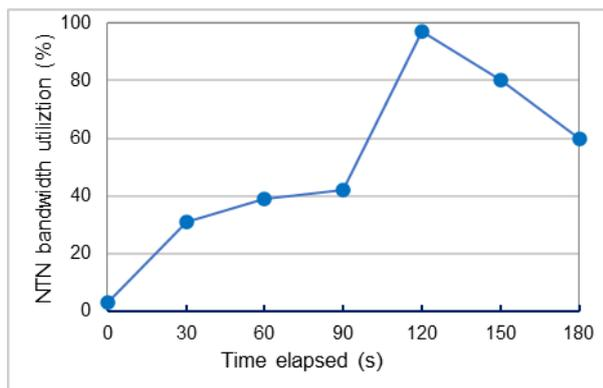
(a) NTN bandwidth utilization versus experiment time. When network congestion is created by injecting background traffic from around 60 seconds, the NTN bandwidth utilization surges to nearly 100%. The utilization decreases after increasing the NTN bandwidth by the control decision made by the INCA controller.
