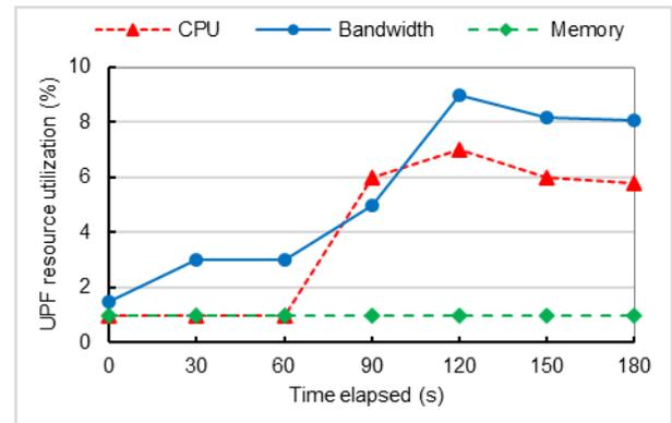
(b) UPF's resource utilization versus experiment time. The bandwidth and CPU utilization of the UPF increase from 60 seconds due to the background noise traffic. However, as the utilization is still very nominal, the INCA controller decides nothing to do with the control of CPU, bandwidth, and memory resources.
