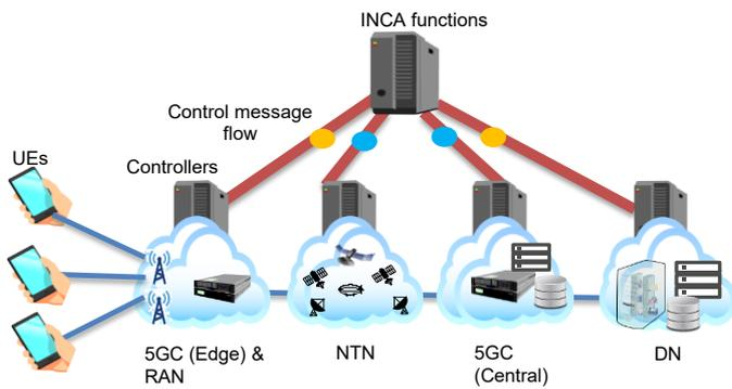
Figure 4 - End-to-end network topology and control message flow.
