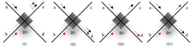
**Figure 1** – The four possible combinations when two indistinguishable photons arrive at 50:50 BS.
