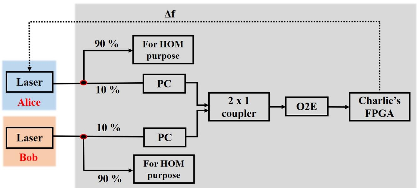
**Figure 3** – Block representation to achieve frequency overlap between photons from independent sources.
