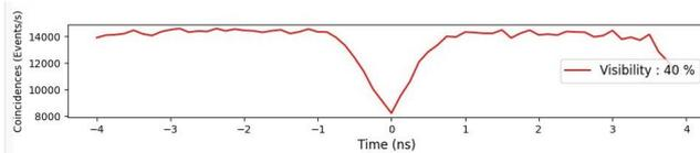
**Figure 8** – Coincidence counts versus time representing the Hong-Ou-Mandel dip.
