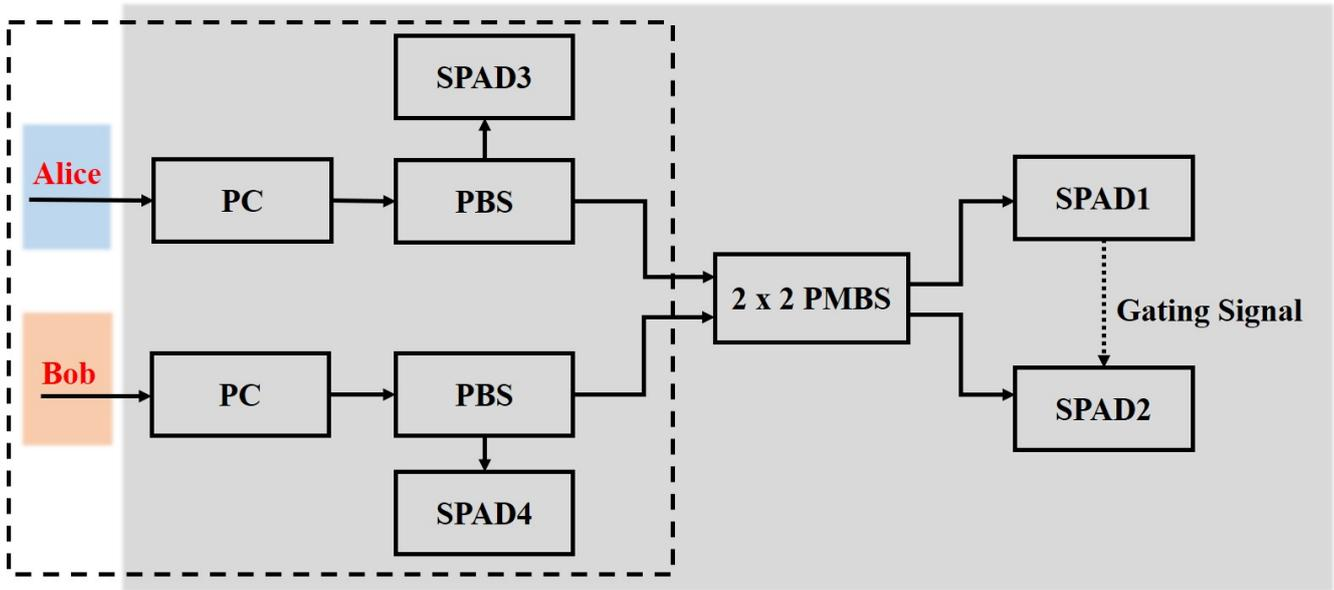
**Figure 4** – The dashed block in the figure represents the setup to achieve polarization overlap between two independent photons.
