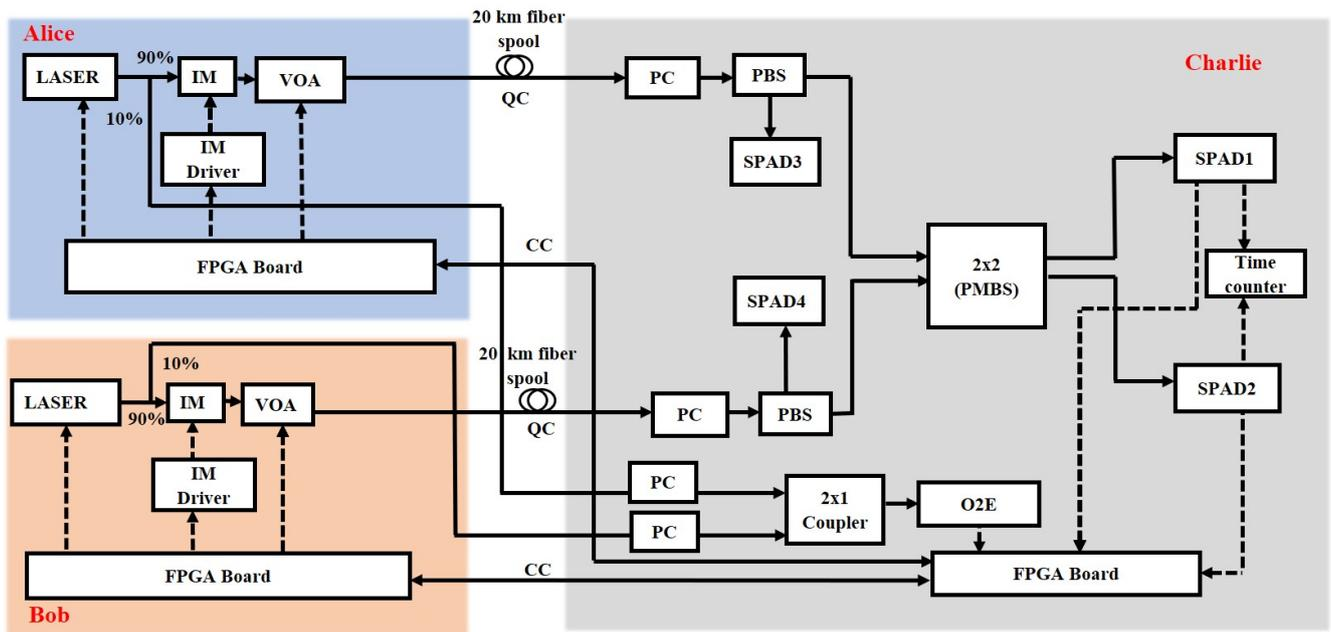
**Figure 2** – Schematic of HOM experiment. Here, PC: polarization controller, PBS: polarizaing beam splitter, PMBS: polarization maintaining beam splitter, SPAD: single photon avalanche photodiode, VOA: variable optical attenuator, IM: intensity modulator, QC: quantum channel, CC: classical channel. Solid lines represent optical connections and dashed lines are for electrical connections.
