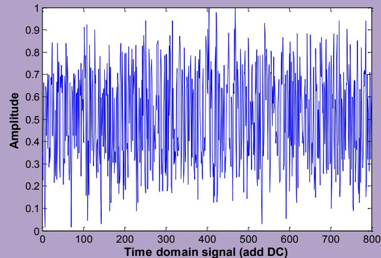
Light intensity must be *unipolar* and *non-negative*. Directed circuit (DC) should be added.
